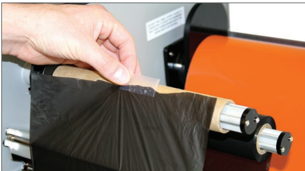
Ribbon being taped to front of supply core
