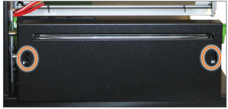
Remove the recessed screws, shown inside the circles.
