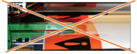
Incorrect: End of media sensor not centered over printable area
