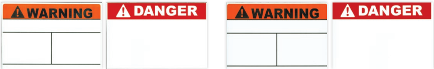
Die-cut and B Mark labels cut correctly (l) ... and cut off-center (r)
