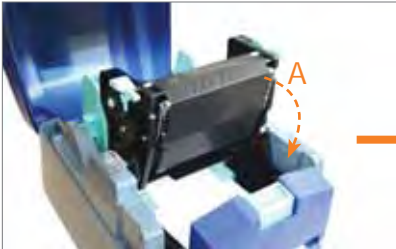
Print carriage in up position
