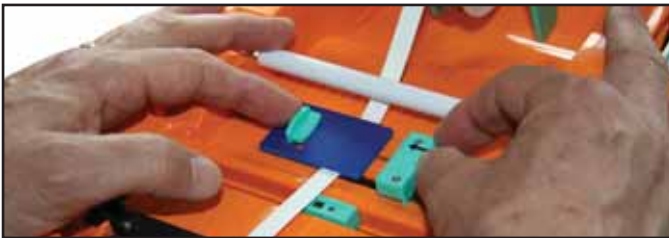
Fig. 6 Shrink tube fitted underneath and in the grooved section of the Tape Guide
