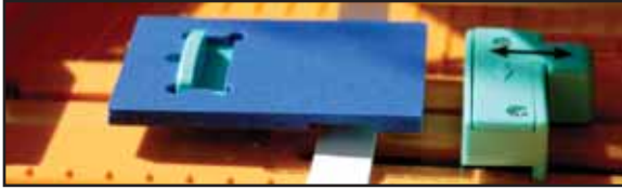
Fig. 5 Tape Guide not completely pressed down with shrink tube aligned under grooved section of Tape Guide
