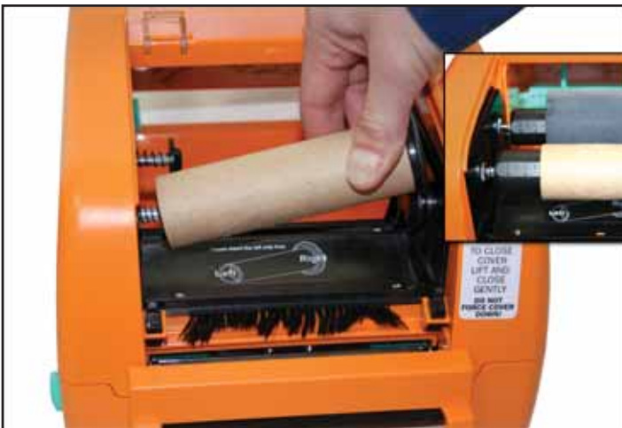
Fig. 8 Ribbon Rewind Spindle with paper core (4.3") being applied to the Front Spring-loaded Hub
