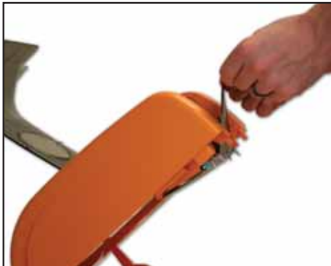
Fig. 12 Ribbon Supply being pulled up to the Ribbon Rewind Spindle
