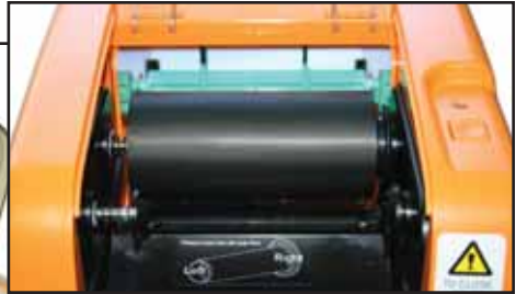
Fig. 7 Ribbon Supply (4.3") Spindle inserted at Rear Hubs
