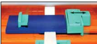
Fig. 7 Adjustable Label Guides pressed together, holding the Tape Guide in place with shrink tube aligned properly over the Media Sensor and fitted in grooved section of the Tape Guide.
