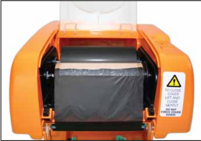
Fig. 13 Ribbon Supply (4.3") taped to Ribbon Rewind Spindle
