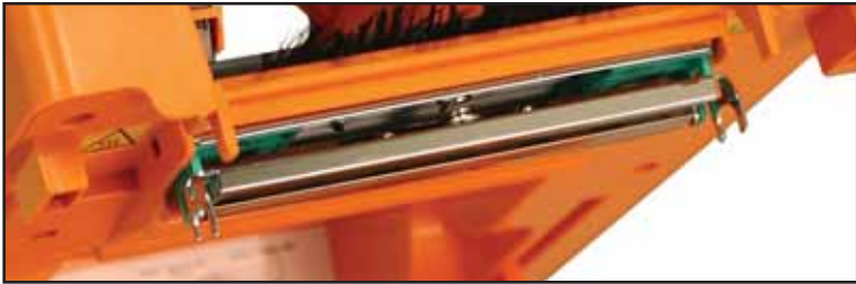
Fig. 1 Print Head is the entire metal bar that sits under the top printer cover
