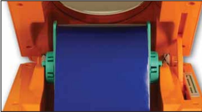
Fig. 2 Loaded Label Supply Spindle set in Label Roll Mount slots
