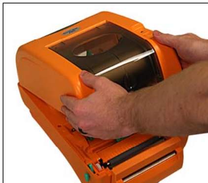
Fig. 3 Use both hands to close the top cover
