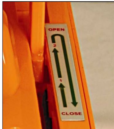
Fig. 1 Top cover support is fixed at position 2
