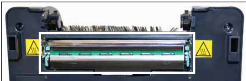
Fig. 2 The entire area outlined in white should be cleaned
