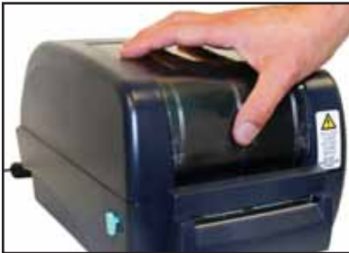
Fig. 1 Press down and in to unlatch
