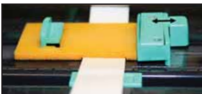
Fig. 7 Adjustable Label Guides pressed together, holding the Tape Guide in place with shrink tube aligned properly over the Media Sensor and fitted in grooved section of the Tape Guide.
