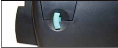
Fig. 10 Printer Release Lever being pulled forward
