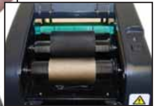
Fig. 9 Ribbon Supply (2.5") Spindles loaded and aligned with each other
