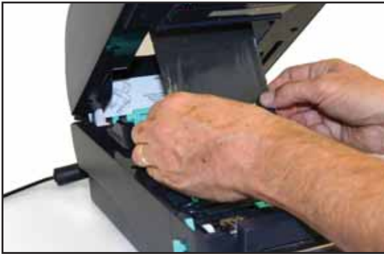
Fig. 11 Ribbon Supply (4.3") being pulled down and underneath
