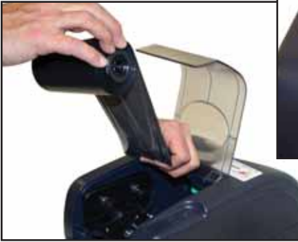
Fig. 6 Ribbon Supply (4.3") spindle being inserted at Rear Hubs
