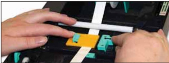
Fig. 6 Shrink tube fitted underneath and in the grooved section of the Tape Guide
