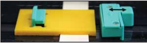
Fig. 6 Tape Guide pressed down into place and over shrink tube supply.
