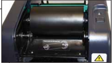
Fig. 7 Ribbon Supply (4.3") Spindle inserted at Rear Hubs
