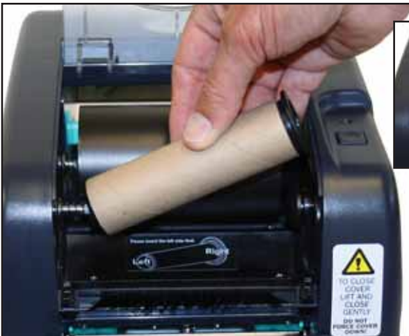
Fig. 8 Ribbon Rewind Spindle with paper core (4.3") being applied to the Front Spring-loaded Hub
