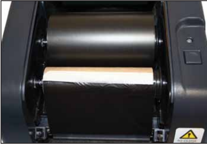
Fig. 13 Ribbon Supply (4.3") taped to Ribbon Rewind Spindle
