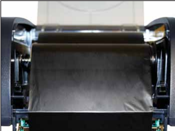
Fig. 14 Ribbon Supply (4.3") rolled tight with dull-side facing out (dull-side of ribbon should face label stock)
