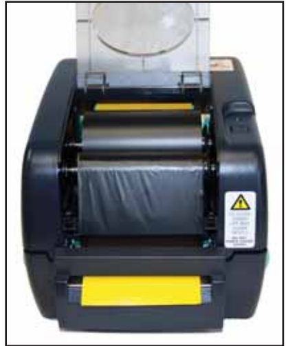
Fig. 7 Printer Cover closed with Ribbon Mechanism Cover open
