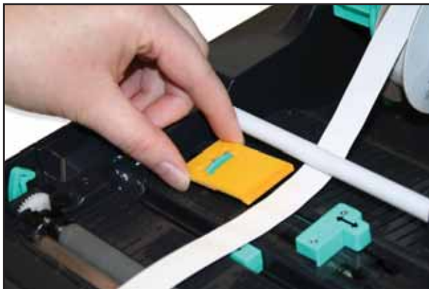
Fig. 5 Tape Guide being fitted over the left Adjustable Label Guide
