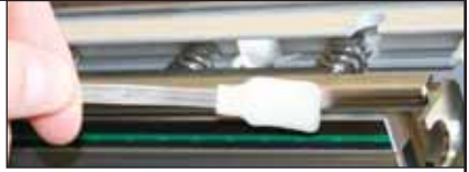
Fig. 3 The front of the print head should be cleaned to remove any ribbon residue
