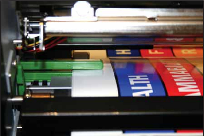
Fig. 10 End of Media Sensor centered over printable-area of RTK Color Bar Die-Cut label
