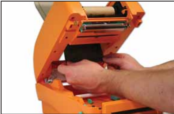
Fig. 11 Ribbon Supply (4.3") being pulled down and underneath
