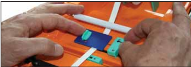
Fig. 6 Shrink tube fitted underneath and in the grooved section of the Tape Guide
