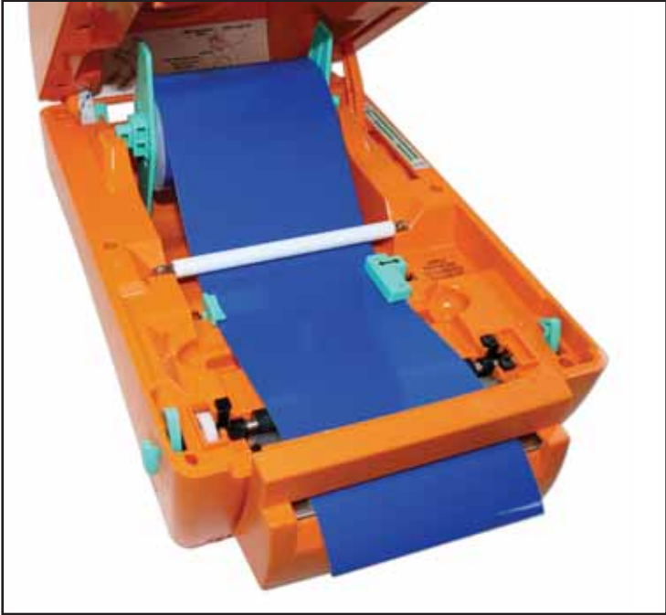
Fig. 4 Label Stock loaded correctly with printable surface faced up and liner faced down
