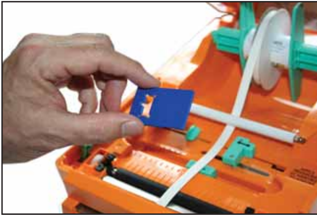
Fig. 4 Tape Guide with smooth, flat-side up, grooved-side down with cut-out opening on the left side
