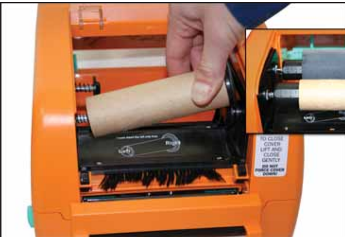
Fig. 8 Ribbon Rewind Spindle with paper core (4.3") being applied to the Front Spring-loaded Hub
