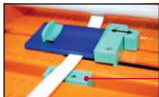
Fig. 6 Shrink tube fitted underneath and in the grooved section of the Tape Guide
