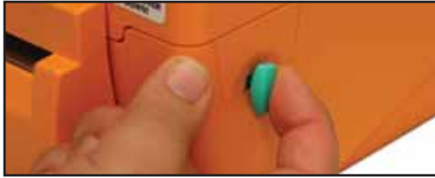
Fig. 10 Printer Release Lever being pulled forward
